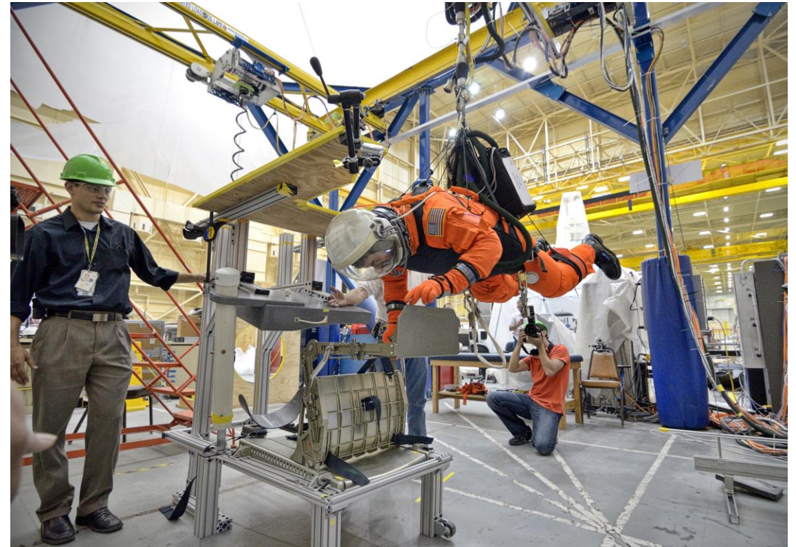
Rail-based suspension system: The NASA Active Response Gravity Offload System (NASA)
